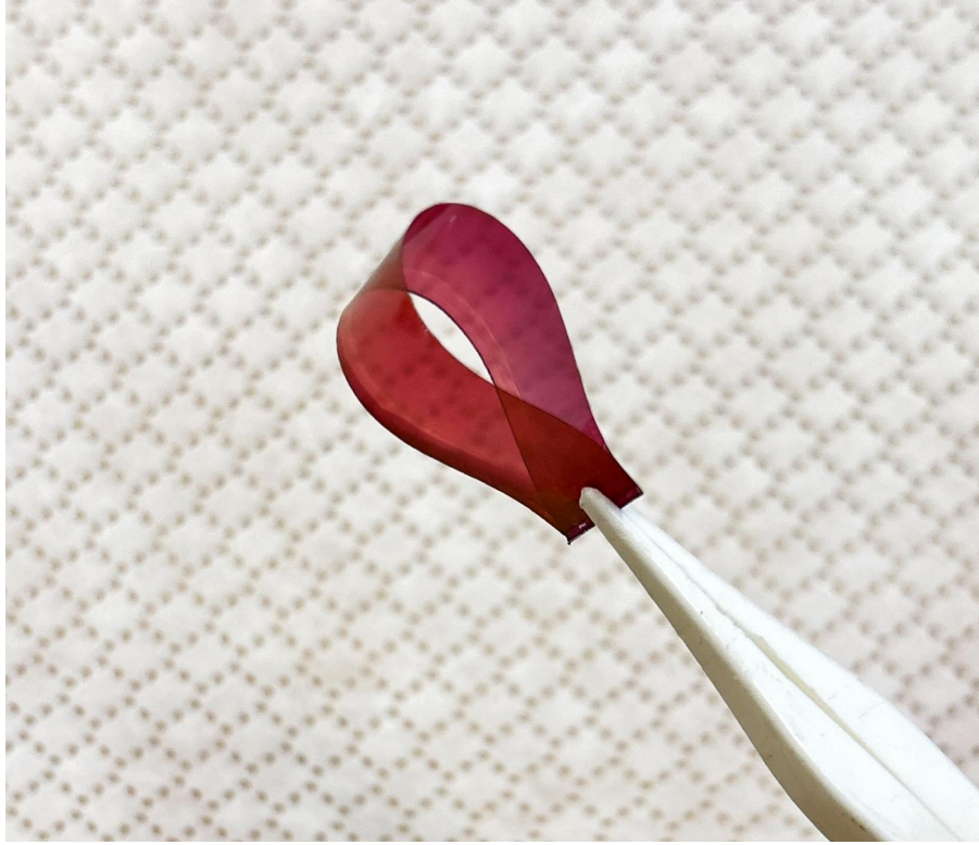
Figure 9.1: A flexible P3HT film annealed at 75°C coated on a flexible PET substrate
